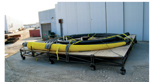
DeepFlex riser on a transportation carousel
